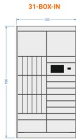
31-BOX-IN steering module V - 18 (61x655x260 mm) S - 9 (440x655x93 mm) M - 2 (440x655x201 mm)
