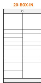
20-BOX-IN additional module S - 14 (440x655x93 mm) M - 3 (440x655x201 mm) L - 3 (440x655x417 mm)
