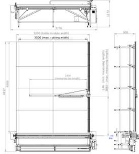
Table of basic dimensions of US-1 cutting tables depending on the selected table module length (for max. cutting width 2000mm)
