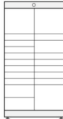
20-BOX-IN additional module S - 14 (440x655x93 mm) M - 3 (440x655x201 mm) L - 3 (440x655x417 mm)
